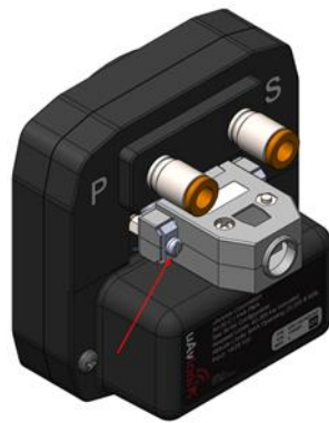
Figure 14 - AV-Link Backshell Connector Removal
