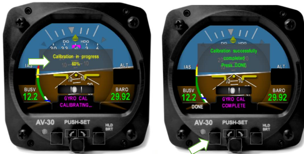
Figure 30 - Gyro Calibration Procedure
